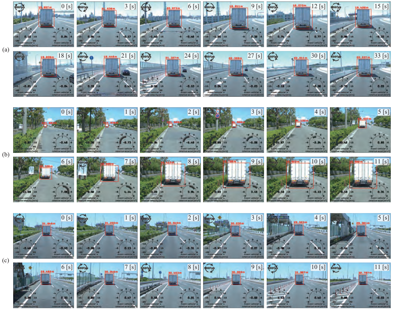
Fig. 6. Tracking results of (a) approaching and leaving, (b) sudden throttle and braking, and (c) intensive vibration. The red rectangle denotes the bounding box in tracking using A-MOSSE. The bounding box is labeled with the estimated distance. The relative velocity and acceleration are shown at the bottom left and right, respectively. All results can be found in the supplemental video.
