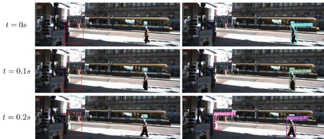
Fig. 6. (a). Test results using blind spot pre-detection method (left). (b). Test results by directly applying YOLO to entire images (right)
