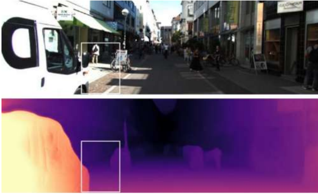
Fig. 3. An example of Monodepth2 inference and detected blind spot
