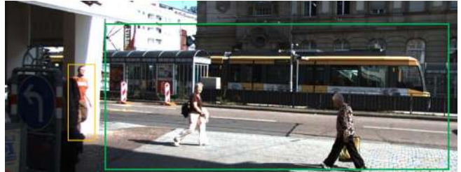
Fig. 1. Different regions in the same image. Image region can have sudden pedestrians (orange), and region can be neglected (green)
