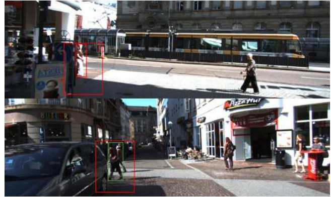
Fig. 5. Examples of pedestrian detection and danger level analysis
